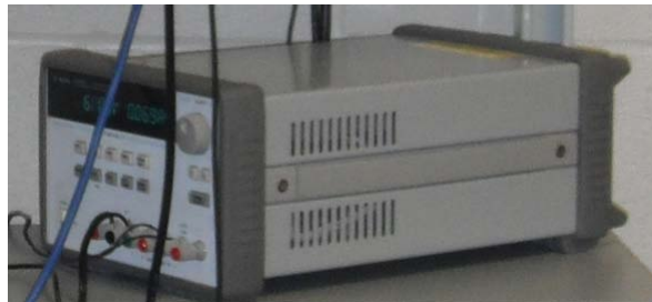
Figure 22. Power supply to Active EM Probe
